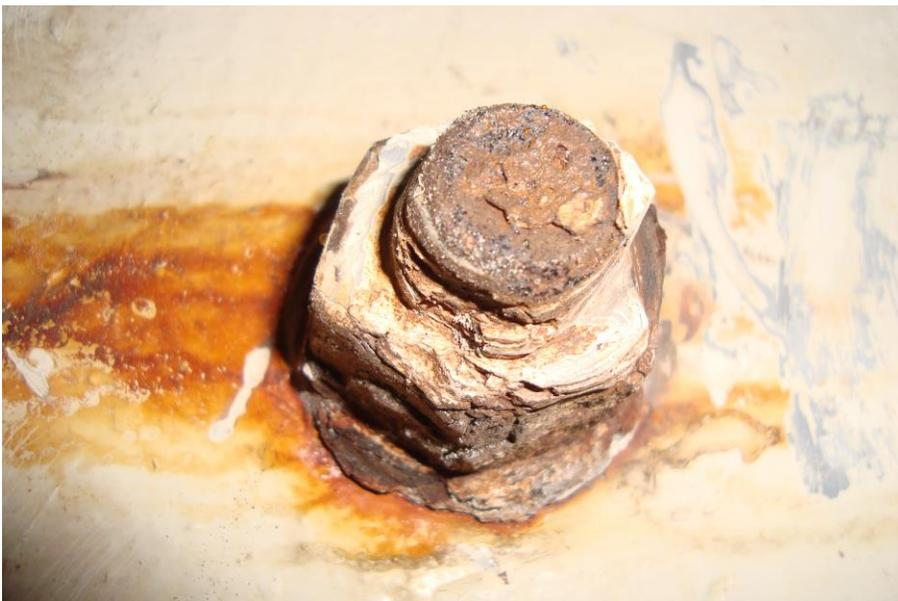
Metal deck fairs little better and often the corrosion origin is at fastener penetrations. The interaction between the hot work steel of case hardened self-tapping screws and the cold worked deck steel as well as the galvanizing is a corrosion cocktail once acids (like chloramine) or salts are introduced.
