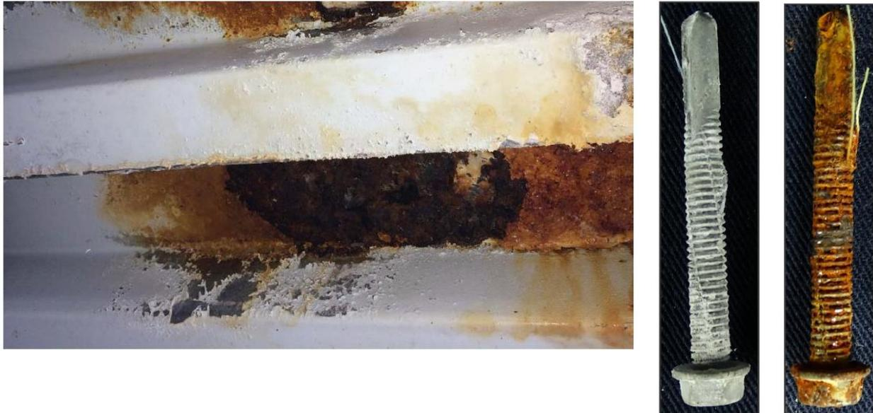
But we use corrosion protected screws to fasten down our gypsum sheathing and insulation boards – surely those will be ok! Right? The manufacturers give us test data that say they are good for 3000 hours? Well yes ... and no. Let's look at the way they get tested and how we use them.
